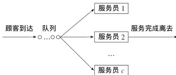
图 10.3  $c$  个服务员,一个公共队的图解表示
